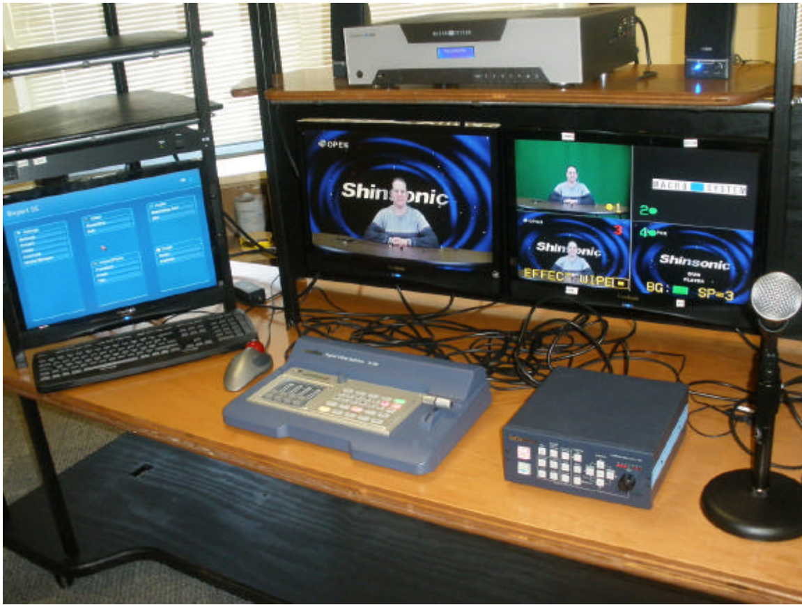
View showing: Datavideo SE-500 switcher, Datavideo Chromakeyer, Casablanca Editor (top center) , Program monitor, Preview monitor, Casablanca editor monitor (left) and voice-over mic.
